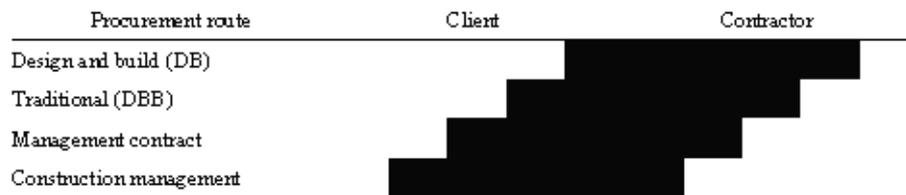
Figure 1: Schematic chart on risk transferring and distribution [31]
